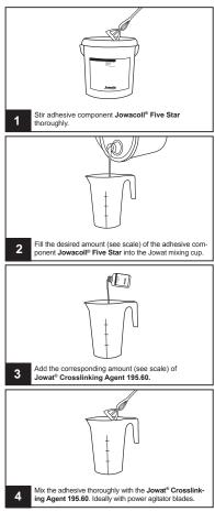
Mixed adhesive must be used up as fast as possible, at the latest after 120 minutes. Remaining adhesive must be disposed according to the Safety Data Sheet and the Jowat mixing cup has to be cleaned thoroughly.
